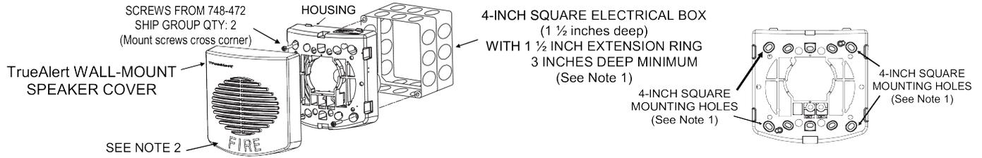
Figure 5: A4902-9716, A4902-9717 TrueAlert Wall-Mount Speaker Mounting
