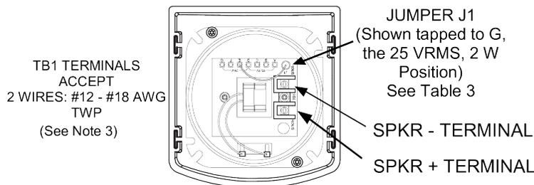
**Figure 4: TrueAlert Wall-Mount Speaker Configuration (Rear View)**
