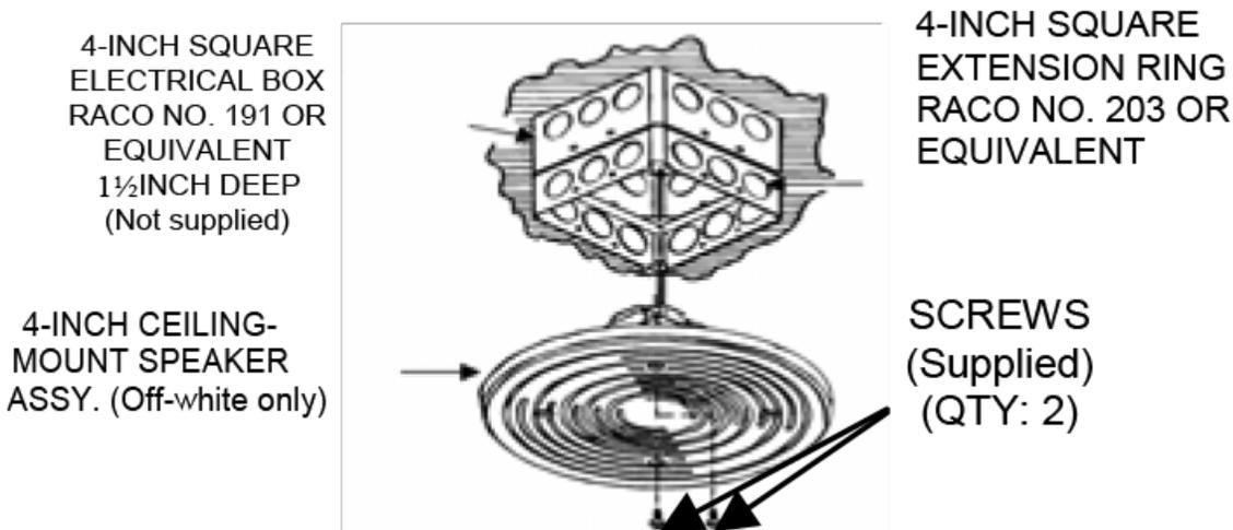
Figure 6: A4902-9721 and A4902-9722 TrueAlert Ceiling-Mount Speaker Mounting
