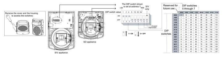
Figure 3: Setting the DIP switch address
