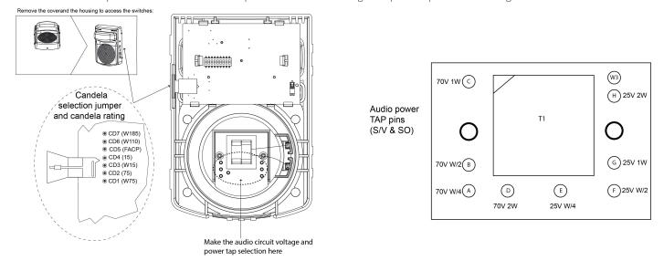
Figure 4: Setting the strobe and appliance configuration
