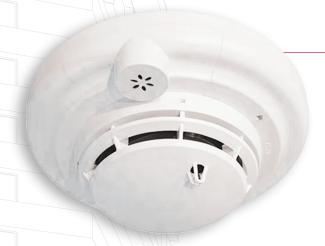
**MULTI-SENSOR DEVICES**. By combining multiple types of sensors (e.g., smoke, heat and CO gas) in a single device, you can protect against a broader range of fire types and gain better immunity to false alarms. The ability to combine up to three sensors in a single device can also save installation and wiring costs.
