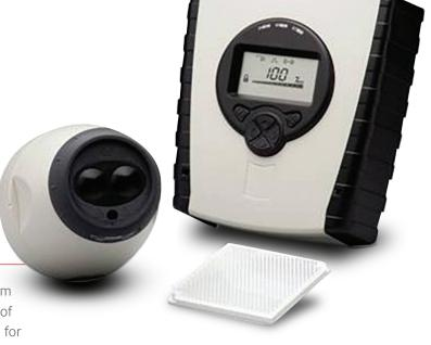
**BEAM DETECTORS.** Beam detectors use a laser beam and a reflector to measure the presence and concentration of smoke across an open area. They are the preferred solution for warehouses, atriums, arenas, and other open areas where it is either impractical or not cost-effective to use traditional point-type sensors or aspirating smoke detection.
