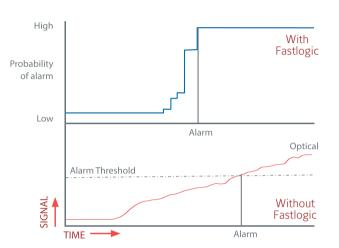
FastLogic calculates that the sensor response indicates a high probability of a fire. In many cases, FastLogic is able to detect fires more quickly and accurately.
