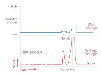
Although the sensor reaches the threshold for long enough to cause an alarm, FastLogic analyzes the signal pattern and calculates a low probability of it being a fire. In this example, FastLogic prevents the initiation of a false alarm.
